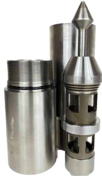
Compared to traditional ESP check valves, the JCV optimizes surface area to maximize force in the up-hole direction during a restart. This enables it to be successful in wellbores where conventional check valves may be permanently checked after a shut down. Furthermore, since the area on the bottom of the inner dart is larger than the top, gas locking concerns that exist in conventional check valves are effectively eliminated.
